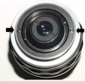
2. You should now be able to unscrew the lens. It's a bit like a continuous focus adjustment. You should end up with 2 pieces like this.
