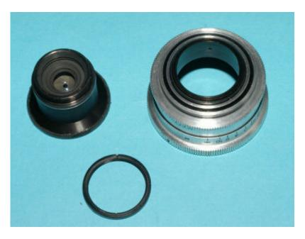
Remove or loosen the 3 screws around the front rim of the focus ring on the main body unit. The ring can now be unscrewed and cleaned if needed.
