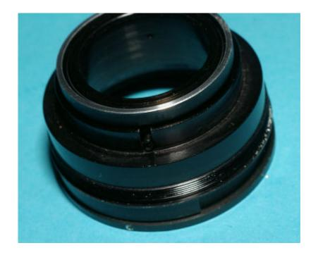
Note the position of the hole for the guide pin. It should look the same on the other side. You may want to screw the inner section fully home and mark the 2 parts the make sure you start the helix in the right place. Remove, the inner helix and then all three parts of the focus unit can go off to be degreased.
