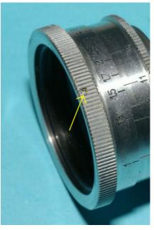
Have a good look at this picture. Note the position of the stop pin and how close to the rim of the middle section, the outer part comes. Remove the screw and if you try the focus again, you will see that the 2 rings "lock" together just past this point. When you re-assemble this part, there are many start positions for this fine helix and this is the one you are looking for.
