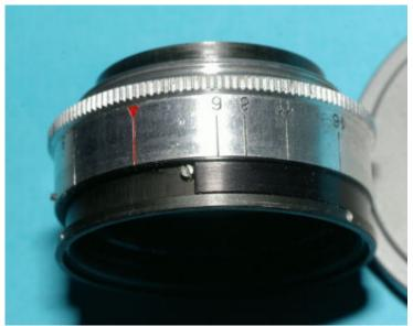
Remove the limit pin (light blue) if you haven't already done so. Remove, the lock screw shown by the red arrow. The outer casing/lens mount can no be unscrewed, cleaned and put to one side.
