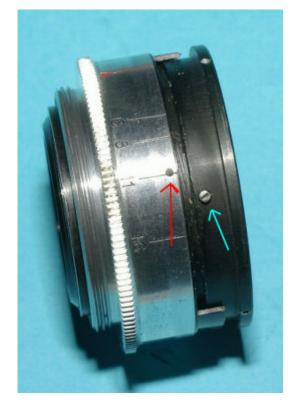
Remove the 2 guide pins, the one shown here and the other one on the opposite side. The outer part of the focus unit can now be removed.
