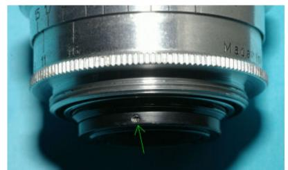
If the diaphragm is difficult or sticky to turn, remove the guide pin. If not put the lens unit to one side.
