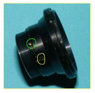
Both parts can now be carefully cleaned. To re-lube this part, I use a lithium-based grease that is a bit thicker than the silicon based grease used on the helix. The arrow shows the important part. It is this rubbing on the main body that gives the diaphragm it's "feel". By using a thicker grease, I find the ring is smooth to turn but less likely to get knocked out of place whilst focussing. Use a little to start with and add more till you get the right feel for you.
