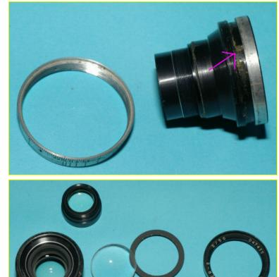
The trim ring and front element should now drop out and you should have a set of parts like this.
