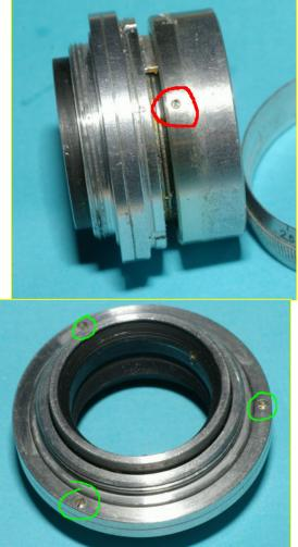
Remove the 3 screws around the front part of the body and remove.
