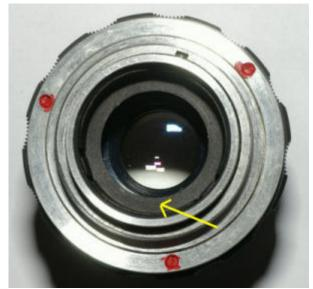
Remove the 3 screws around the focus ring and remove the ring.
