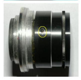
Using a pair of ground pliers or a lens spanner, remove the rear-retaining ring and unscrew the ring. As you start to unscrew it, the lens unit will become loose so you will need to support it from the front. Once it is slack, you should be able to unscrew to lens unit from the front. Put it safe to one side.
