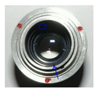
Remove the 3 screws shown here locked by red paint (It was a "new" lens after all!). Lift off the rear retainer ring.
