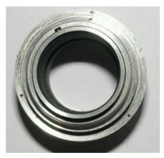
Have a good look at the focus helix. It has one of four start positions and it is important to get the right one or the lens will not focus correctly. You may want to mark the position as shown here by the yellow circle. If not, note how the alloy body ring almost touches the focus helix as it touches the limit pin. Having done that, remove both the limit pin and the guide pin shown in the photo. Note that the guide pin is slightly shorter than the limit pin.
