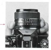
5. Keep this lever down for open-aperture exposure reading. (Lens aperture stays fully open, and stops down to pre-selected f/stop as you depress shutter release.) Move it up for depth-of-field preview or for stop-down exposure reading. (Lens aperture actually stops down to pre-selected f/stop.)
