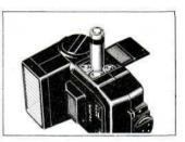
Insert four batteries, plus (+) and minus (-) ends correctly as illustrated in the Battery Compartment, then replace the cover by sliding it in until it locks.
