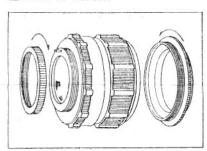
This Reverse Adapter consists of two pieces, RI and R2. One end of RI is screwed into the front of the lens like a filter and the other end is screwed into the Extension Tube or Extension Bellows. R2 is then screwed on to the rear end of the lens (now facing the front). It couples with the lens aperture control pin for adjusting the aperture manually.
