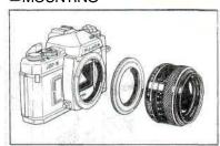
Screw the Fujinon lens into the Mount Adapter X-S. Then place the red dot on the adapter's rear end against the red dot on the camera's lens mount and turn the lens 65' to the right. It will lock into position with a click.
