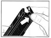
Open the Battery Compartment Cover by lifting both ends up slightly and pulling it toward you.
