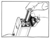
② Insert four penlight batteries (AA size) as shown in the battery compartment and replace the cover. ③ If the batteries are not properly loaded or are exhausted, the Auto Winder will not run, or will take longer time to advance the film. In such cases, the batteries should be replaced or reloaded correctly.
