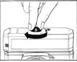
camera, fit the thumbscrew of the winder securely into the camera's tripod socket and turn it tightly.
